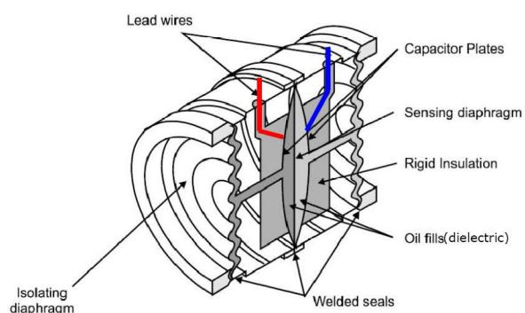
Functional scheme of the differential pressure sensor
